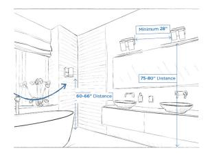
For two bowl vanities, fixtures should be mounted directly above each bowl and should be spaced a minimum of 28" apart.
